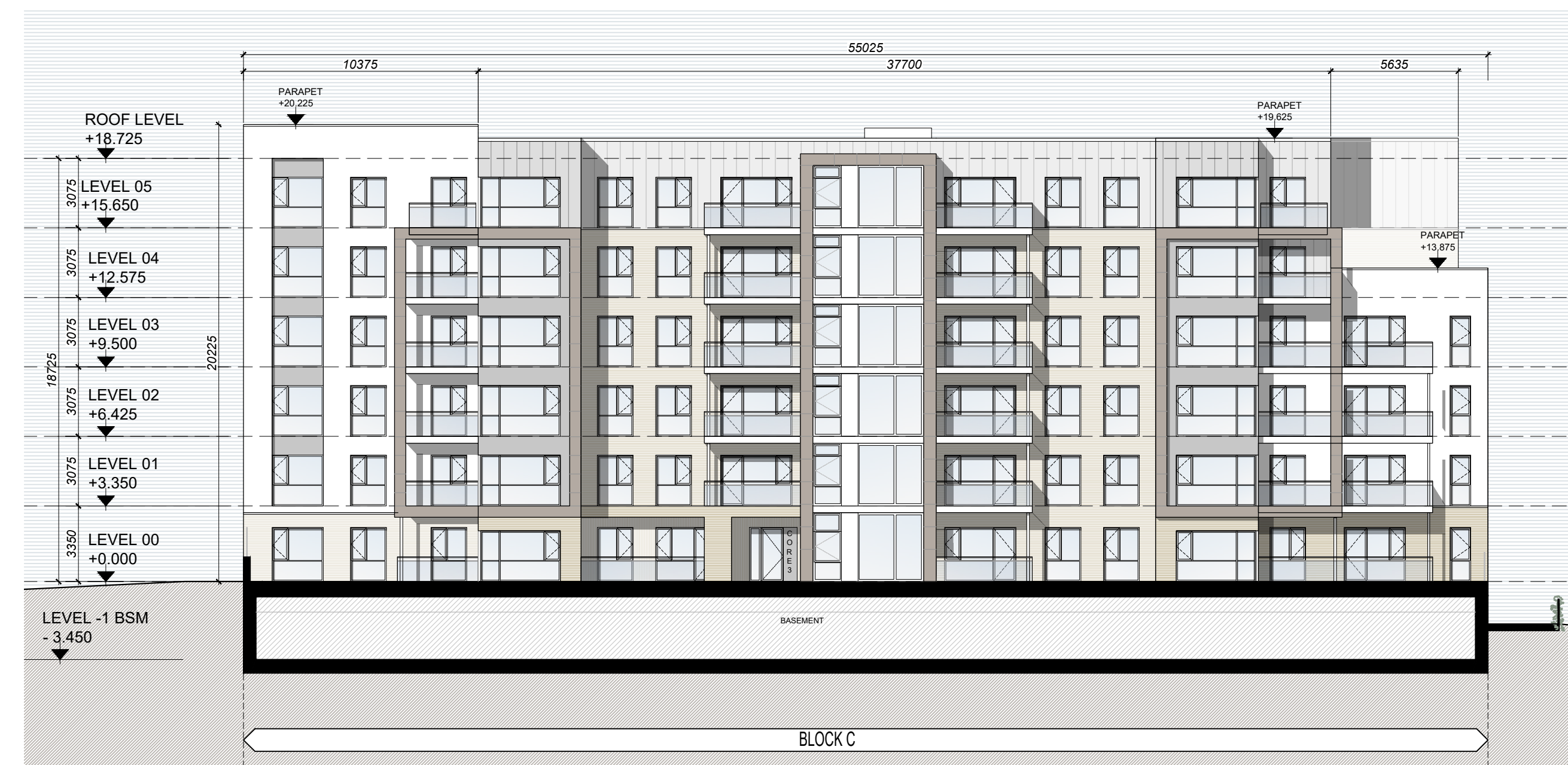
BLOCK C - EAST ELEVATION - 09
